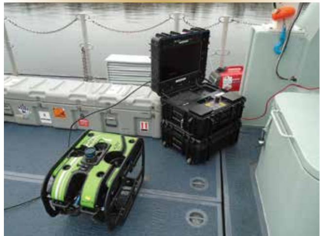
Tools like Teledyne's SeaBotix ROV (above) and Deep Trekker Inc.'s DTG2 ROV (below) allow technicians to easily survey the condition of a ship's underwater hull.
