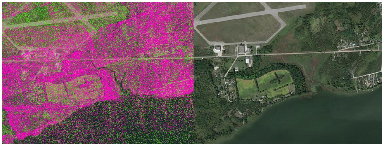
Figure 119: For sites covered by LEAP dataset, point classification is not reliable to identify laser pulses that hit water surface. Here, points in pink are classified as water (class 9) and green, as ground (class 2). On the right, satellite image of the same sector.
