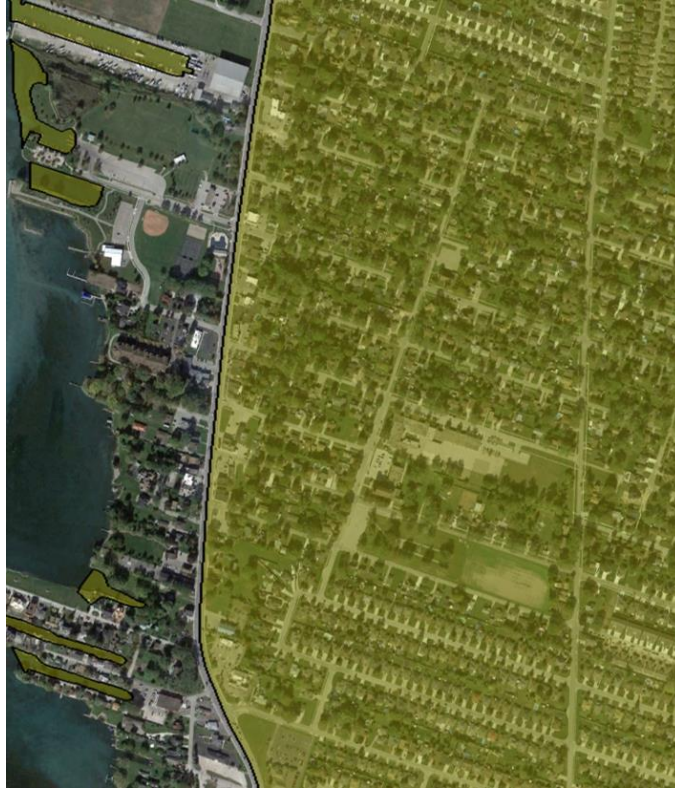
Figure 112: In Detroit River Marsh (12DRM), upland area from the road is mostly anthropogenic. Therefore, it was assumed that the road would act as a dyke and areas upland have been masked (yellow).
