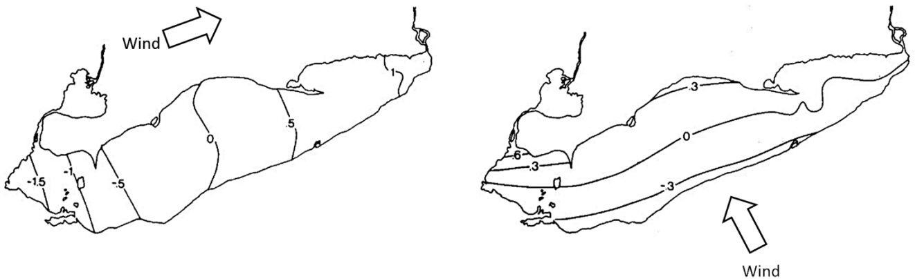
Figure 20: Steady wind set-up (in m) for a wind stress of 1.0 Pa in Lake Erie. Left panel: longitudinal response. Right panel: transverse response. After Hamblin (1987).
