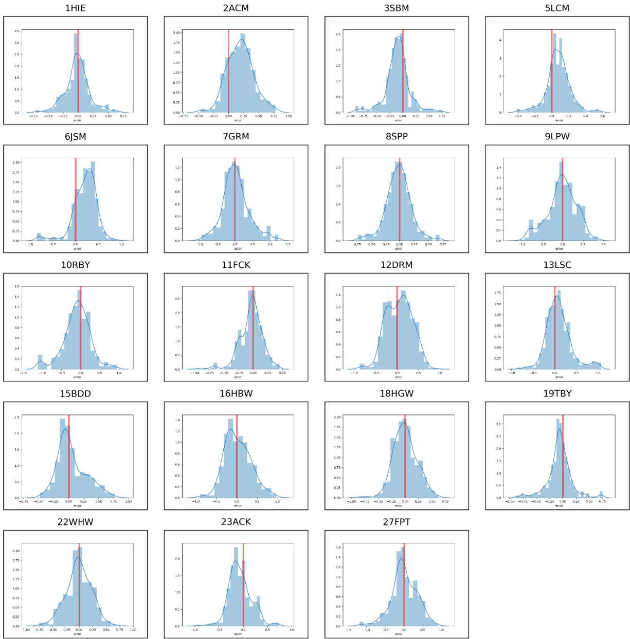
Figure 133: Distribution of DEM's elevation error for the 19 study sites 27 . Most sites have a distribution centered on 0 (red line). Only sites where the LIDAR correction method was less effective (2ACM, 6JSM) still have a positive elevation bias (curve shift to the right).
